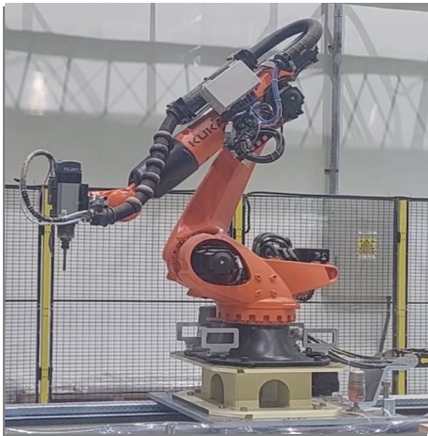
Fig. 2. Experiment setup of the KUKA ROBOT for milling operation (Milling was performed by the KUKA ROBOT manually after that the process was done with the AI proposed method)
